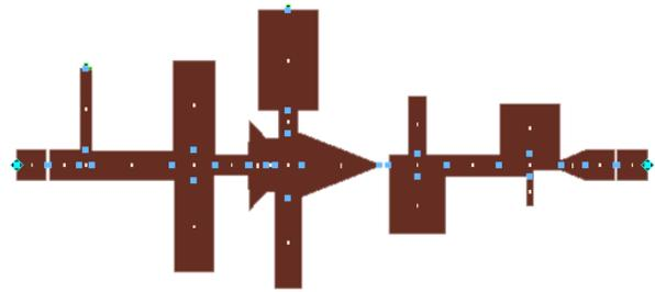
Figure 2: RF circuit developed and optimized for the CGHV14250F transistor (shown in yellow) with HB ADS module for one of initial PCB variants having 70  $\mu\text{m}$  thick lamination and 3.18mm thick CuFlon substrate.
