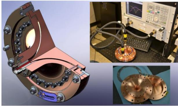
Figure 3: [LEFT] combiner/divider CAD model, [RIGHT] testing the prototype device and the prototype disassembled.
